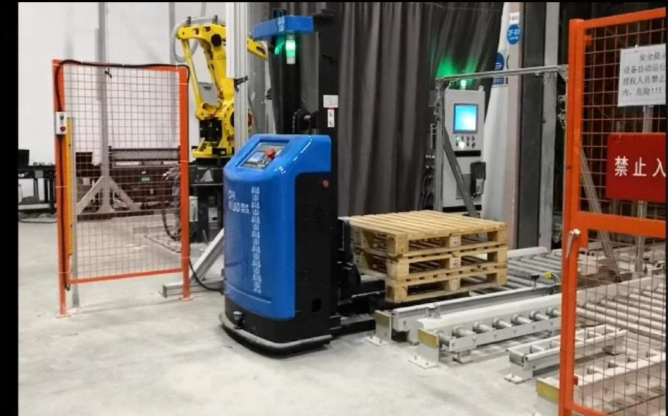
➤ Automatic forklift Automatic forklift connect the AS/RS and transport cart
